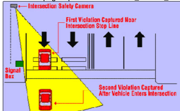
Figure 3-2: Typical intersection safety camera set up ( http://www.winnipeg.ca/police/safestreets/is_camera_tech.stm )
